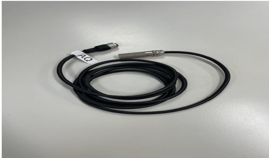
Figure.12 - Air quality probe
